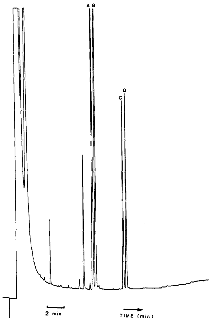
Fig. 1. Capillary gas-liquid chromatogram of diastereomeric derivatives (with MTPA chloride) of methyl-2-hydroxypalmitate (A, B) and methyl-2-hydroxystearate (C, D). Column (25 m \times 0.32 mm I.D.) coated with OV-1; carrier gas helium; column temperature programmed from 180 to 240°C at 2°C/min.
